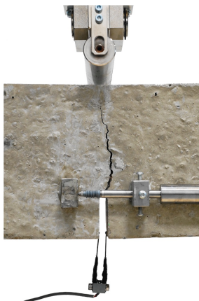
Detail of CMOD testing to EN 14651 with 200kN high stiffness frame 50-C1701/FR. See Additional Information
